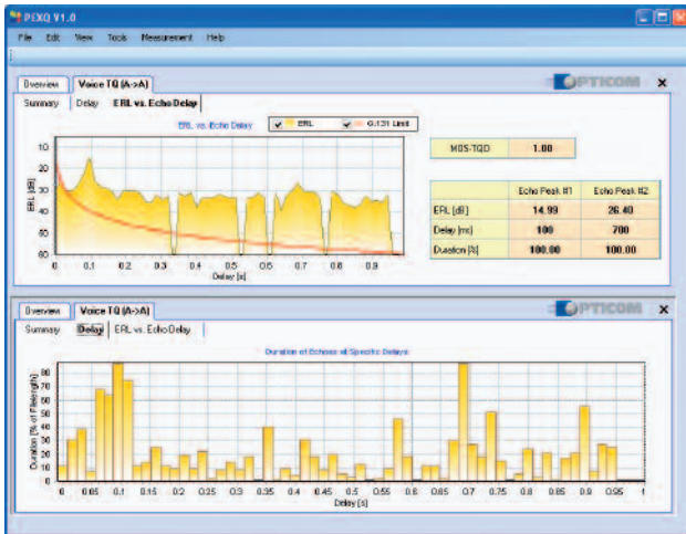
Comprehensive analysis of Talking Quality: Echo Return Loss analysis and PESQ-TQ MOS (upper diagram), Echo Delay Histogram (lower diagram)
