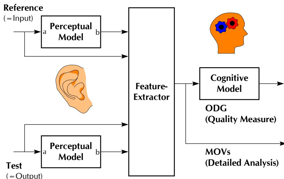
Figure 5: The structure of the generic perceptual measurement algorithm
