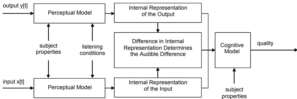
Figure 6: Block diagram of the basic model of the PSQM algorithm [19]
