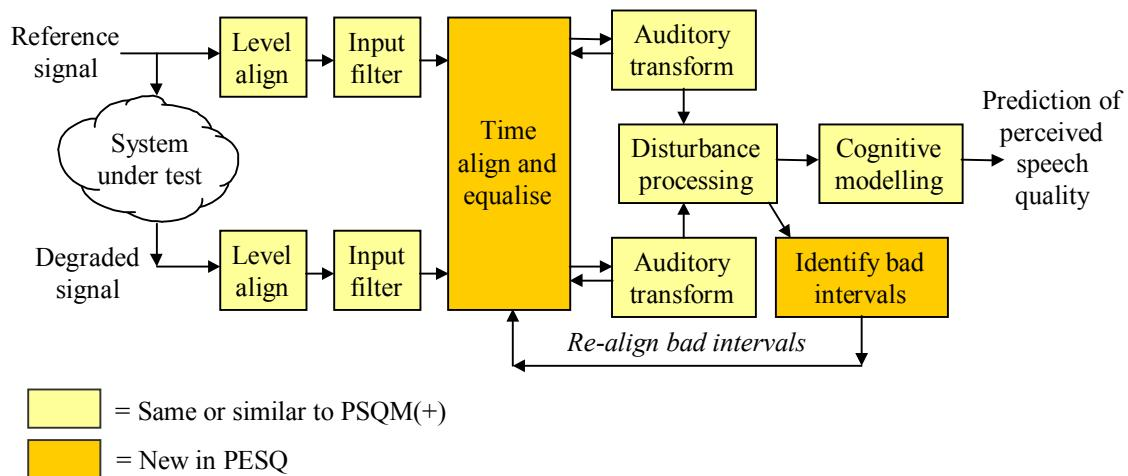
Figure 7: The structure of the PESQ algorithm
