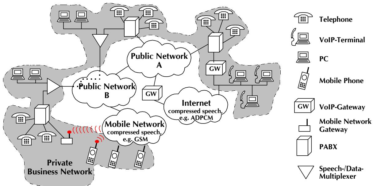
Figure 3: An example for the topology of today's telecommunication networks
